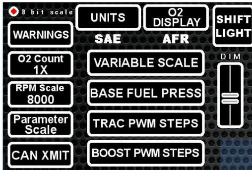
**UNITS** button will allow the user to toggle between SAE and SI units. This applies to temperature, pressure, speed, and distance.
