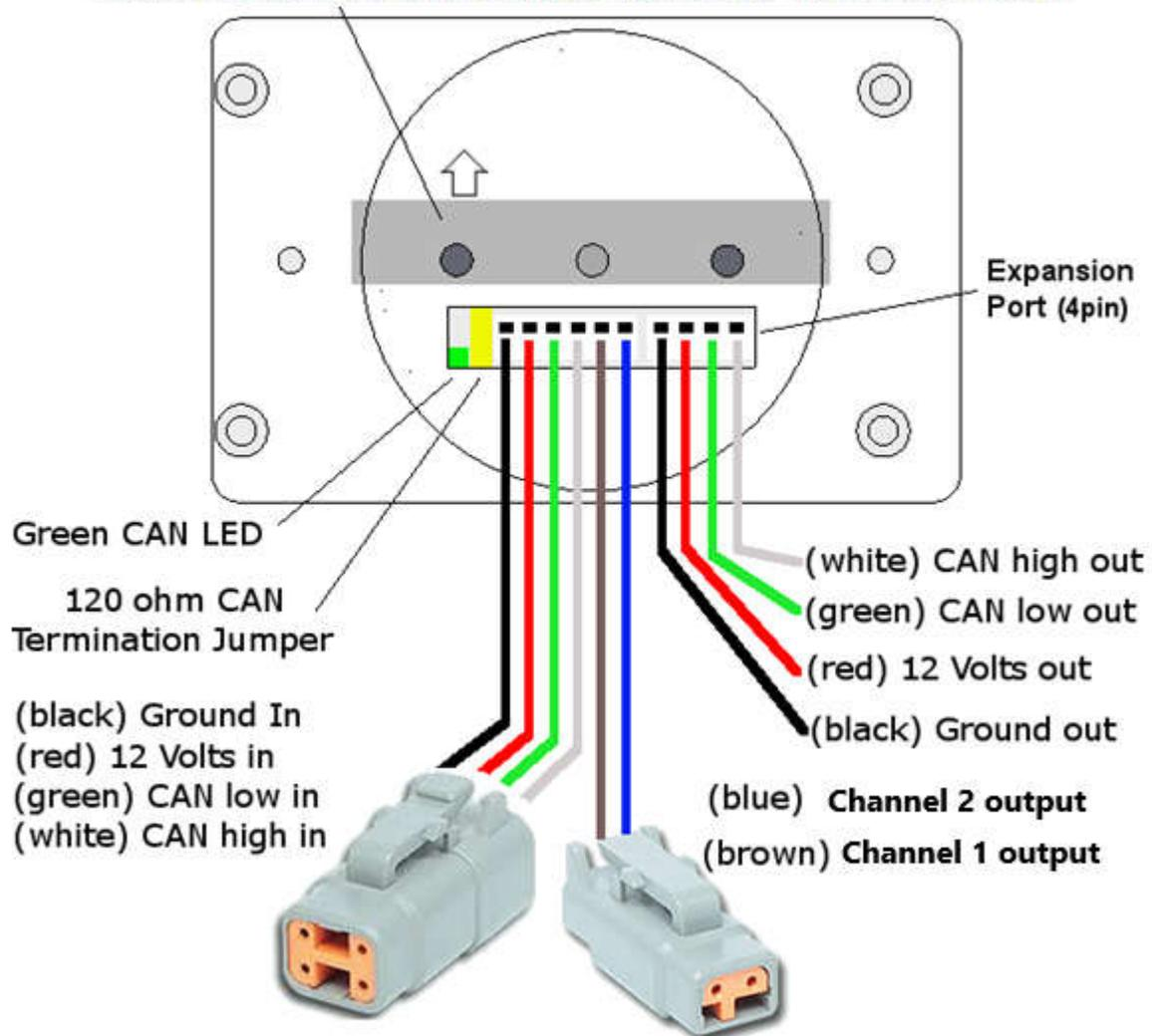
**Data LED:** This indicator will flash whenever the gauge is energized and CAN communications are present. Use this to confirm communications.
