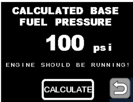
**Base Fuel Pressure:** Use this feature to calculate the base fuel pressure while the vehicle is at normal idle. This will be used on the **Fuel** screen in order to verify proper fuel pressure regulator function (assuming that you are using a rising rate regulator with a 1:1 ratio).
