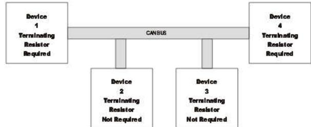
**Notice! This diagram is for the Tyco connectors that are plugged into the Haltech CAN hub:**
