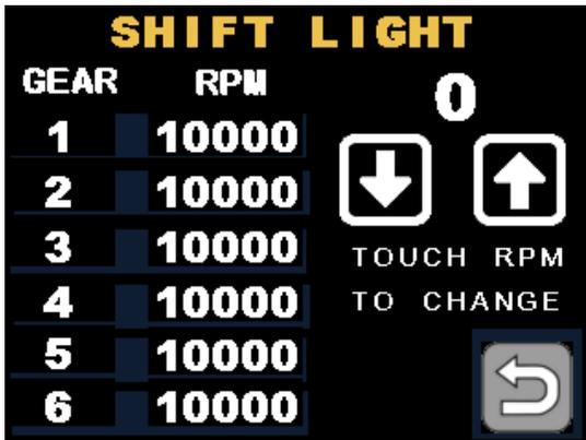
The **Shift Light** functions by RPM per gear. This means that a shift light may be configured in 1<sup>st</sup> gear at 6500 RPM while the Shift light could be illuminated in 2<sup>nd</sup> gear at 7000 RPM if desired. Simply touch the Gear or RPM that you wish to change and adjust accordingly using the arrow keys. Touch the Back arrow to save and the shift light should illuminate while saving.
