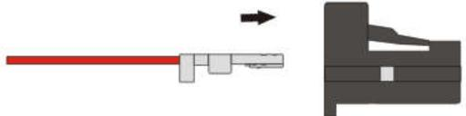
CRIMP PIN TO WIRE AND THEN INSERT INTO BACK OF PLUG WITH THE PIN LOCKING TAB IN THE UNLOCK POSITION. PUSH DOWN TO LOCK PIN IN PLACE
