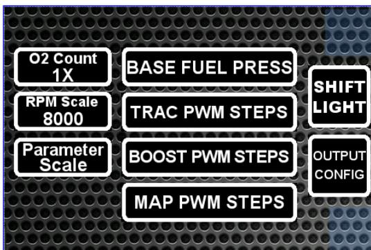
Touching the **Settings** button will allow for Outputs, Shift Light, Base Fuel Pressure, and Output levels to be configured:
