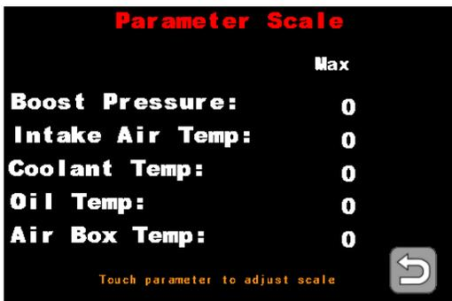
**Parameter scale:** Use this screen to set the maximum range for boost pressure and various temperature slide bars and graphs.
