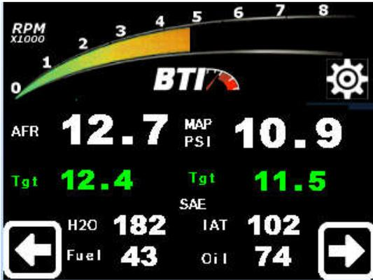
The Setup may be accessed by touching the cog wheel pictured on the top right of the diagram pictured. This is where the Units, Outputs, Boost level, Slip level, Map, Shift Light and output steps may be changed.
