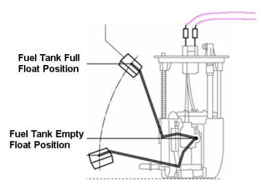
Terminate the Pink wires to the Fuel Tank sending unit. The Sending unit must be isolated from ground or power within the car (just like taking a resistancemeasurementwith a multi-meter) There is no polarity on the pink wires. Consult the vehicle manual to determine the proper wiring. When in doubt, always take your vehicle to a trained professional.
