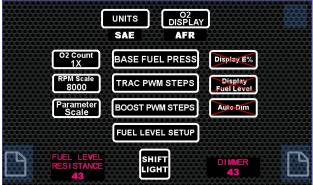
This will bring you into a screen where the Units may be selected, the settings can be accessed, and the shift light may be setup. The Units button will allow the user to toggle between SAE and SI units. This applies to temperature, pressure, speed and distance. The O2 Display button will change how the Oxygen sensor data is displayed. The options are AFR and
