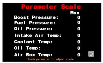
**Parameter scale:** Use this screen to set the maximum range for boost pressure and various temperature slide bars and graphs.
