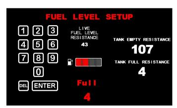
Fuel Level Setup: This is where the fuel level resistance may be programmed in order to take a reading from the fuel level sender. Consult the service manual for the fuel level resistance values.
