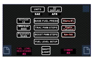
Touch the cog wheel on the touch screen in order to configure the gauge. This will bring you into a screen where the Units may be selected, the settings can be accessed, and the shift light may be setup. The Units button will allow the user to toggle between SAE and SI units. This
