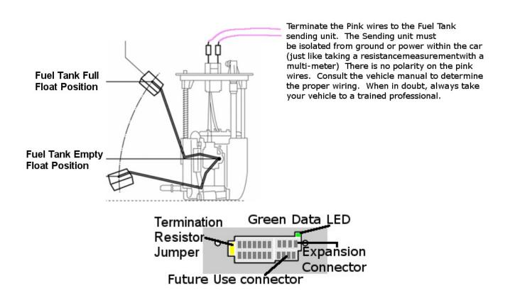
Data LED: (back of the dash) This indicator will flash when ever the gauge is energized and CAN communications are present. Use this to confirm communications.
