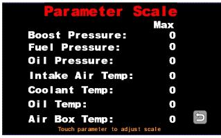
**Parameter scale:** Use this screen to set the maximum range for boost pressure and various temperature slide bars and graphs.
