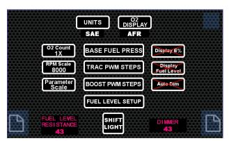
Touch the cog wheel on the touch screen in order to configure the gauge. This will bring you into a screen where the Units may be selected, the settings can be accessed, and the shift light may be setup. The Units button will allow the user to toggle between SAE and SI units. This
