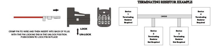
Notice! This diagram is for the Tyco connectors that are plugged into the Haltech CAN hub:
