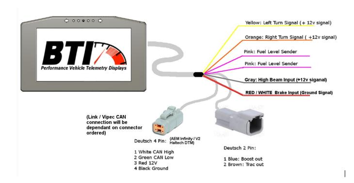
Warning! Ensure that Fuel Level Leads are only connected to the sending unit. Disconnect the sending unit form all other connections including the OEM gauge or ECU!
