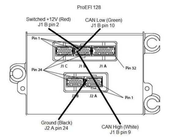
Note: In the event that you have fluorescent lights or neon signs in your vehicle, there is a ground shield wire that is concealed under the heat shrink on the plug and pin harness. The ground shield wire should be connected to ground on one end of the harness.
