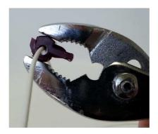
Finally, Plug in the insulated male connector into the T-tap:
