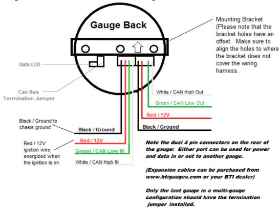
**Dual White 4 pin Connectors:** It does not matter which 4 pin connector you plug the wire harness into. The remaining connector can be used for expansion to more gauges.
