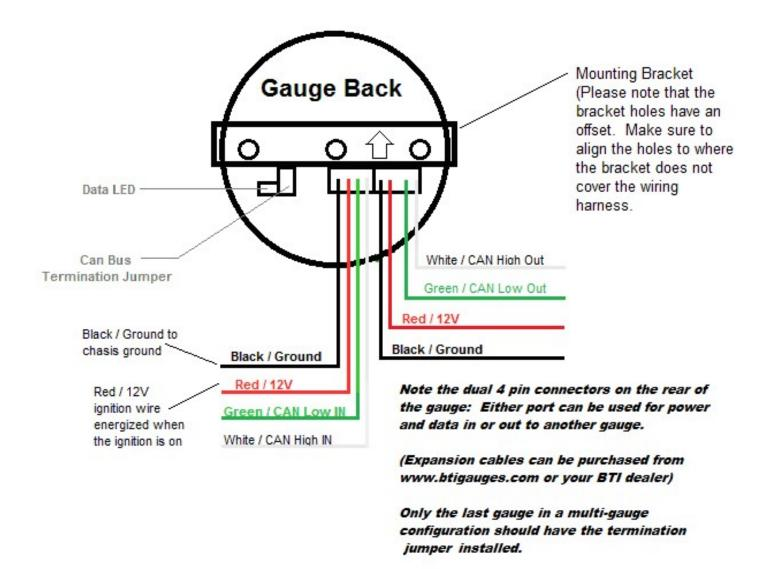
Data LED: This indicator will flash when ever the gauge is energized and CAN communications are present. Use this to confirm communications.
