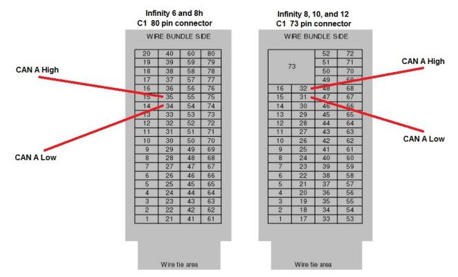
The plug and pin harness has two signal wires (Red and Black). Pin the RED wire to CAN A High and the BLACK wire to CAN A Low on the corresponding connector
