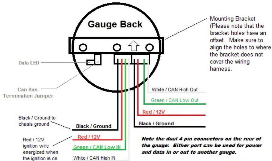
**Note the dual 4 pin connectors on the rear of the gauge: Either port can be used for power and data in or out to another gauge.**
