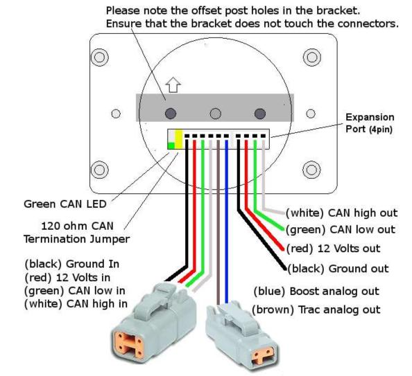
Notice: The gender of the 2 pin plug may be reversed on newer models in order to prevent the improper connection to the "Flash Enable" connector.
