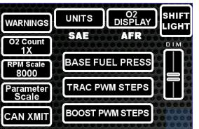
**UNITS** button will allow the user to toggle between SAE and SI units. This applies to temperature, pressure, speed, and distance.
