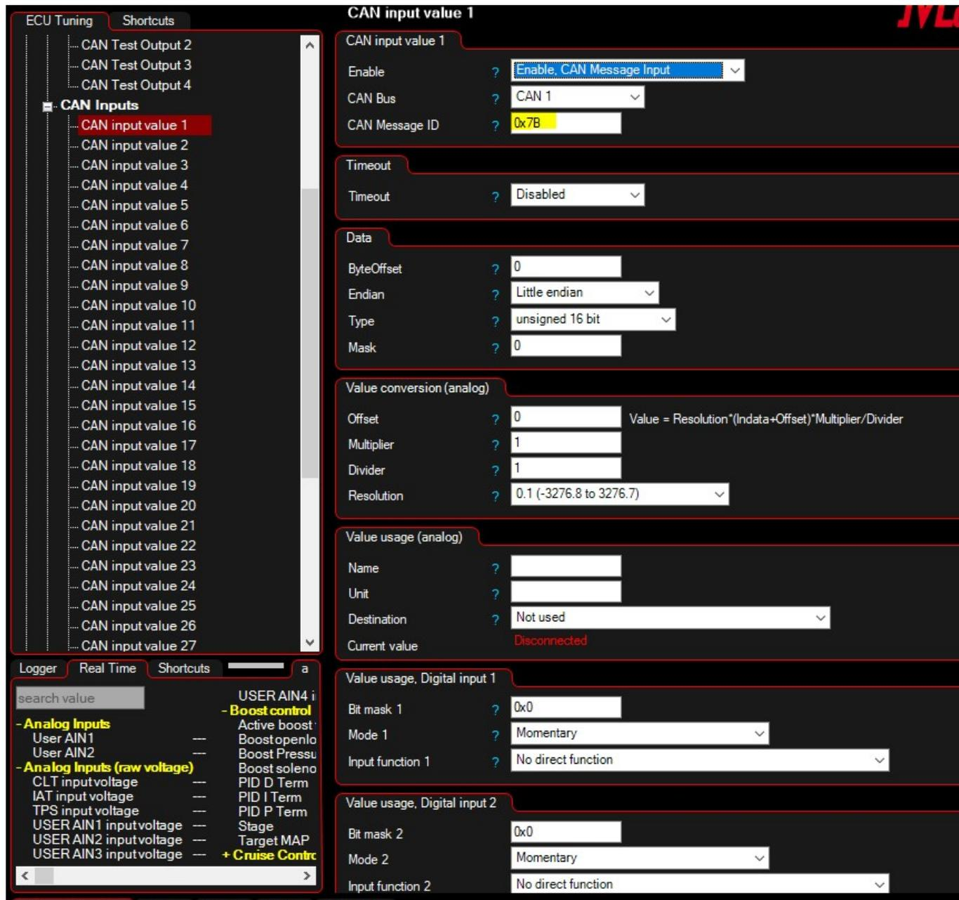
Make note of the CAN message ID as that is configurable in the gauge. The address is configured in the CAN Output screen under the Yellow cog wheel.
