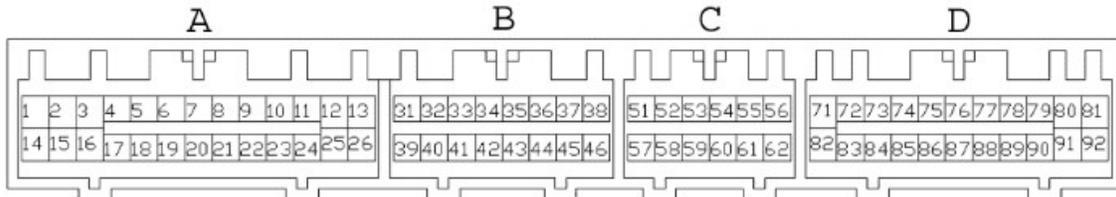
Figure 9: Wire-side view of pinout for 6310 and 6311 EMS
