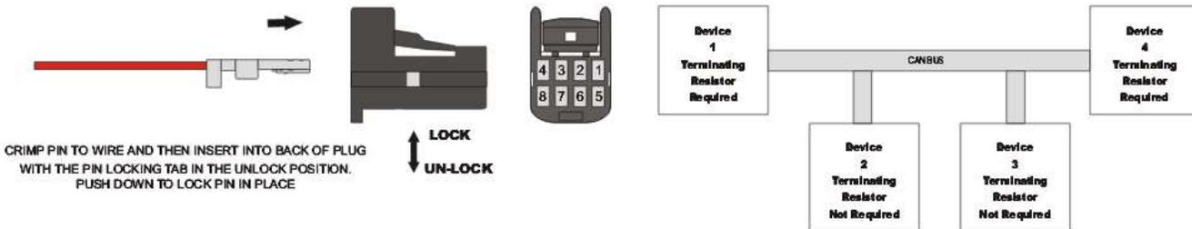
**Notice!** This diagram is for the Tyco connectors that are plugged into the Haltech CAN hub:
