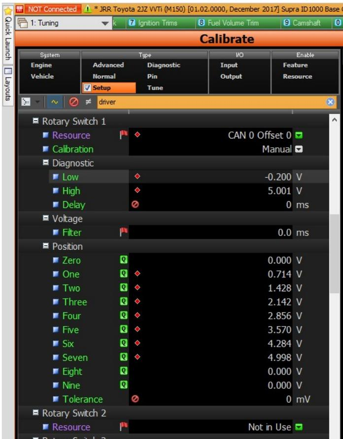
**Example Boost control configuration using Rotary Switch 1.**
