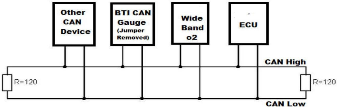
This is what the CAN bus should look like with multiple CAN devices on the bus with the BTI gauge as the last or only device on said bus:
