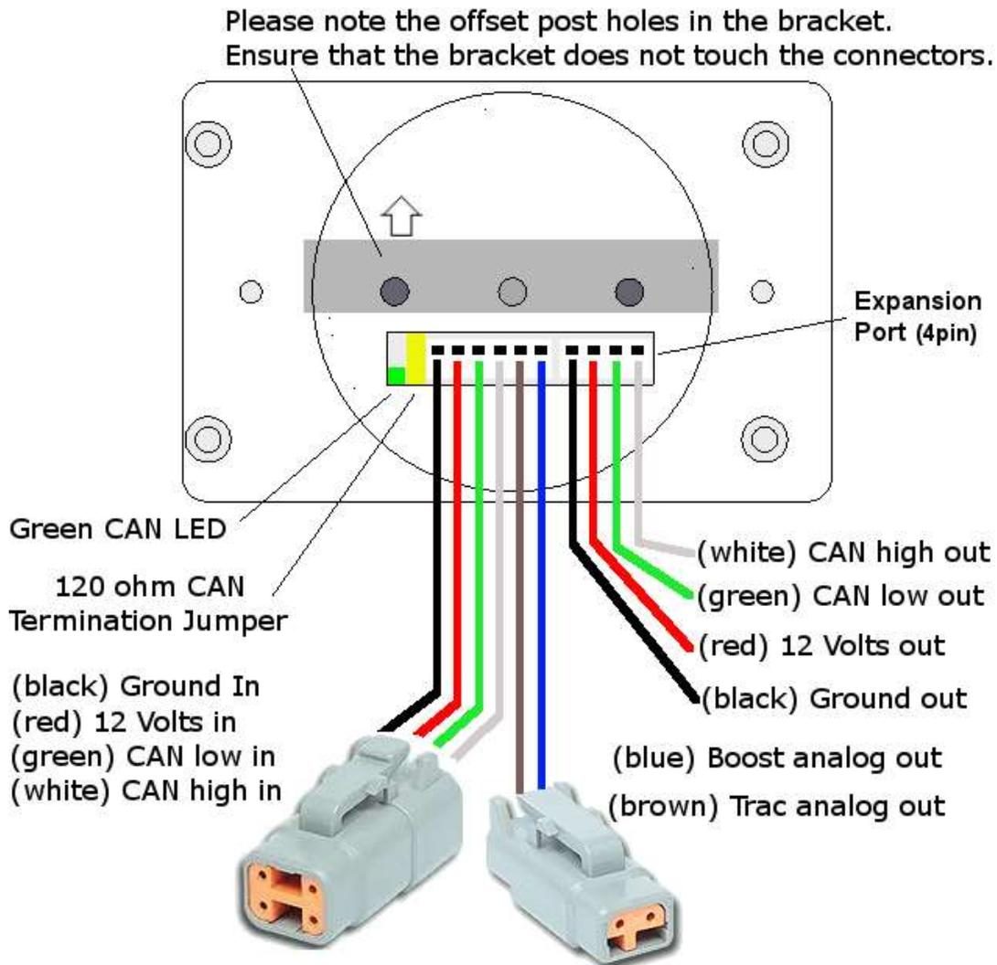
**The wiring is similar for all models. All integrations are shipped with the AEMnet standard DTM connector cable with exception to customers whom selected the Haltech 4 pin DTM connector which is conveniently wired 180 degrees from the**
