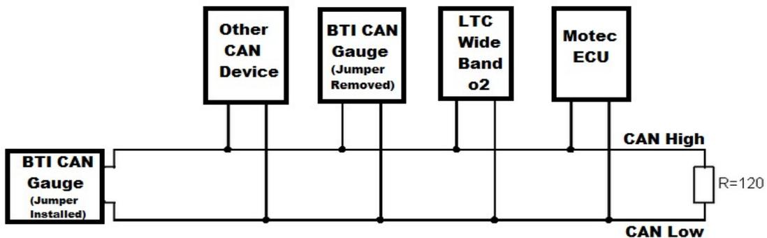
Upon powering up a properly terminated gauge, the Gauge will display the interface and version number.
