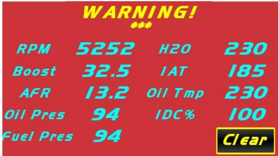
In the event that a user warning does trigger, the warning will be displayed and the parameter highlighted. The warning may be cleared which will cause the display to resume normal operation. There is a warning counter that will re-trigger for a condition that may have been cleared and corrected but the error has reoccurred.
