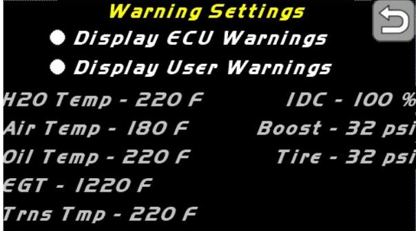
**Display ECU Warnings:** This setting will allow the screen to display warnings generated by some ECUs. Note that not all ECUs generate warnings.
