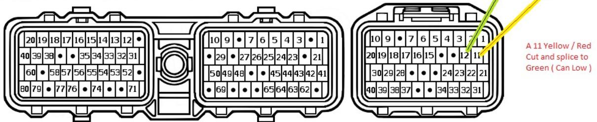
Notice: Not all 2JZ wiring harnesses have pins a 11 and a 12 populated. In the event this should occur, pins or pre-terminated pins with wires are available from Toyota.
