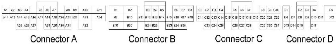
Figure 8: Wire-side view of pinout for 6050, 6051, 6052, 6053, and 6060 EMS
