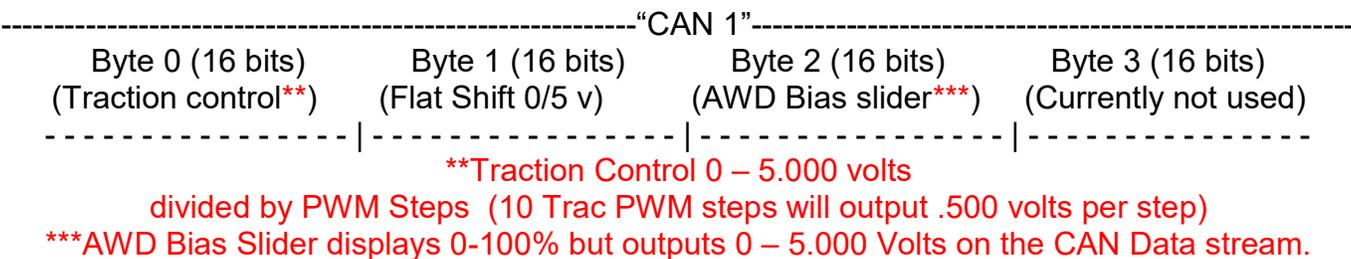
Emtron Tech support has been kind enough to provide these configuration examples in the EMtune software. Emtron support suggests using the CAN address 1400 (578 hex) for data reception from the BTI display.
