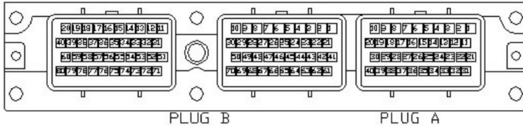
Figure 6: Wire-side view of pinout for 6100 and 6101 EMS
