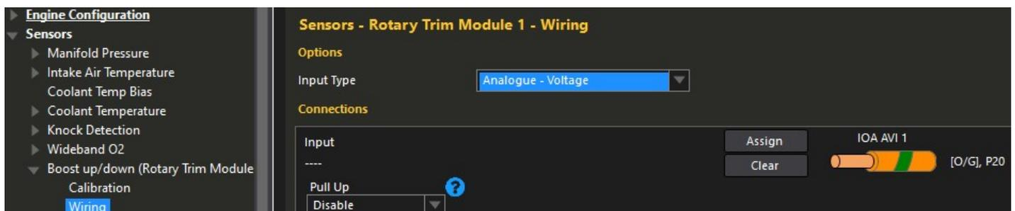
Pictured below is an example of the input selection from the gauge when the ECU is connected to the software. Note that the voltage output from the gauge is visible on the input
