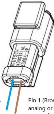
Pin 2 (Blue) 0-5v analog or switched output for channel #2
