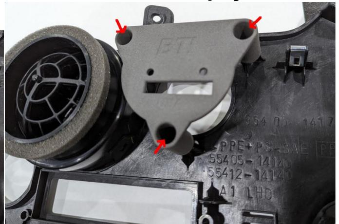
**4. Attach the BTI bracket with the OEM screws. If you do not have these screws, 3 stainless steel screws are included with these display.**
