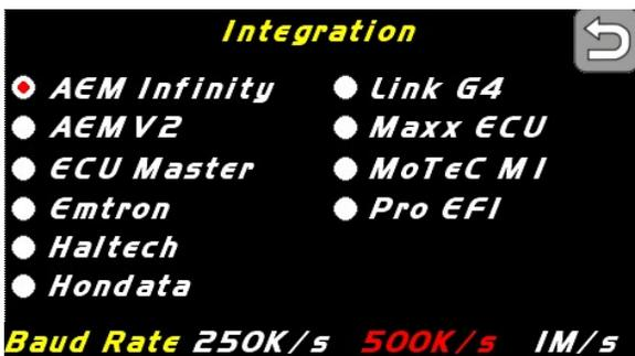
**Integration:** Pressing the Integration button will allow the user to determine which ECU CAN data stream will be received and interpreted by the BTI CAN display.
