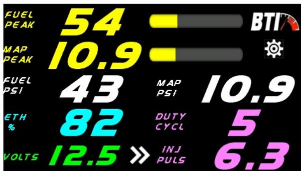
The Base Fuel calculation is used to verify that your rising rate fuel pressure regulator is working correctly as you should see your peak fuel pressure rise with your peak MAP pressure when you are one the Fuel screen.
