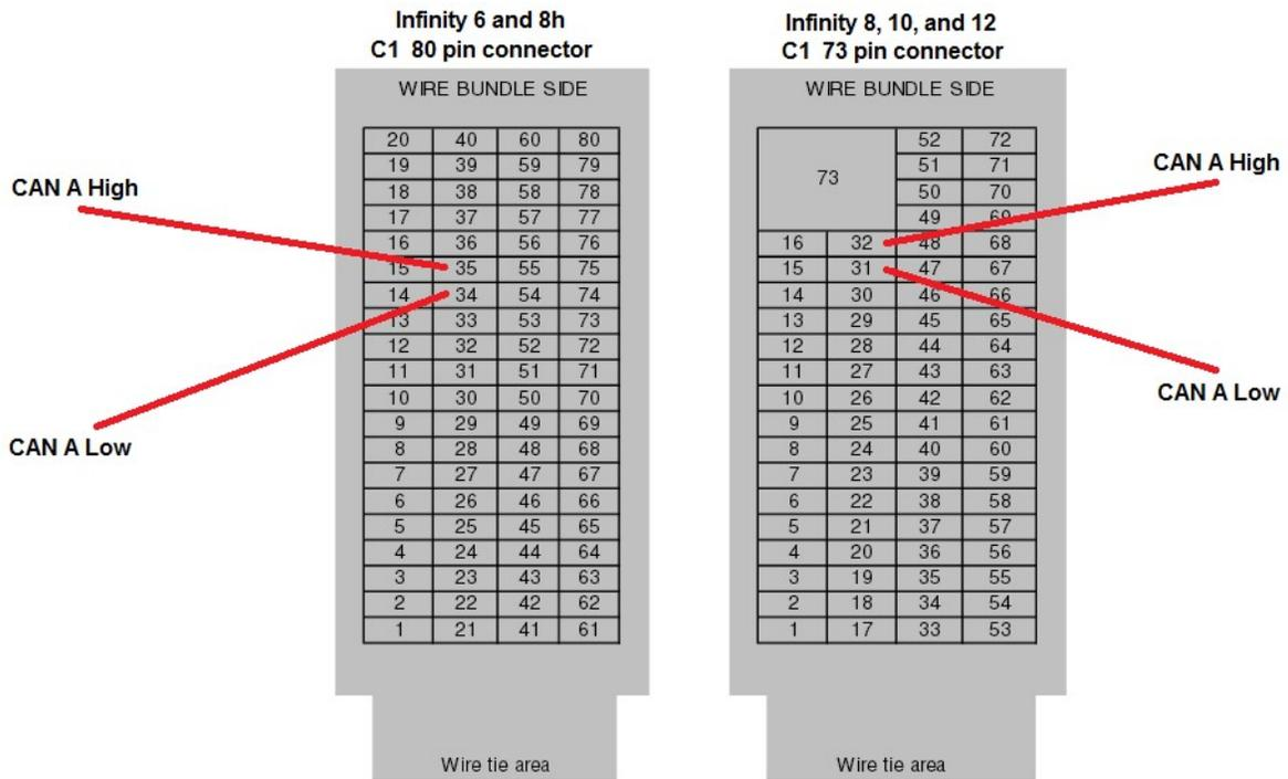
The plug and pin harness has two signal wires (Green and White). Pin the White wire to CAN A High and the Green wire to CAN A Low on the corresponding connector. Connect the Red wire to a switched on / ignition power source and connect the Black wire to ground.
