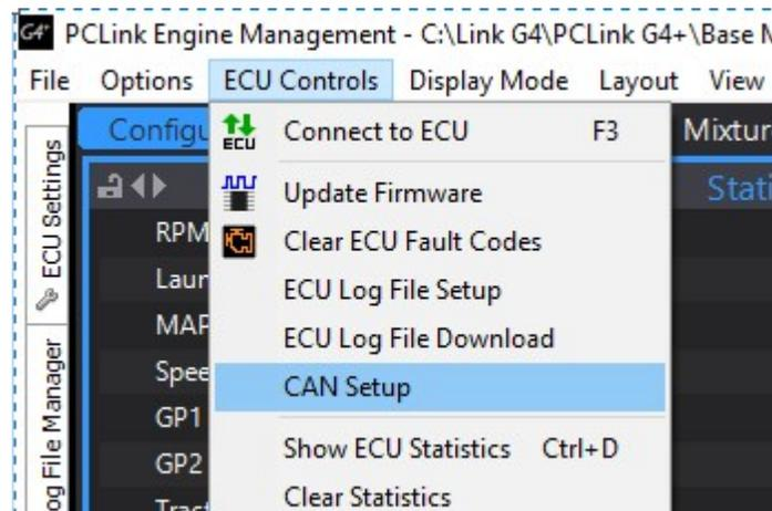
Select the CAN channel that you will be using. “CAN1” or “CAN2” (**Drop in ECUs may be using “CAN 2” if that connector is used for switched power.**)
