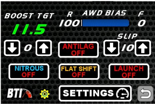
Pressing the yellow cog wheel on this screen will allow the user to set the CAN transmission address. The address is set in decimal, but a conversion to Hex is listed at the bottom of the screen:
