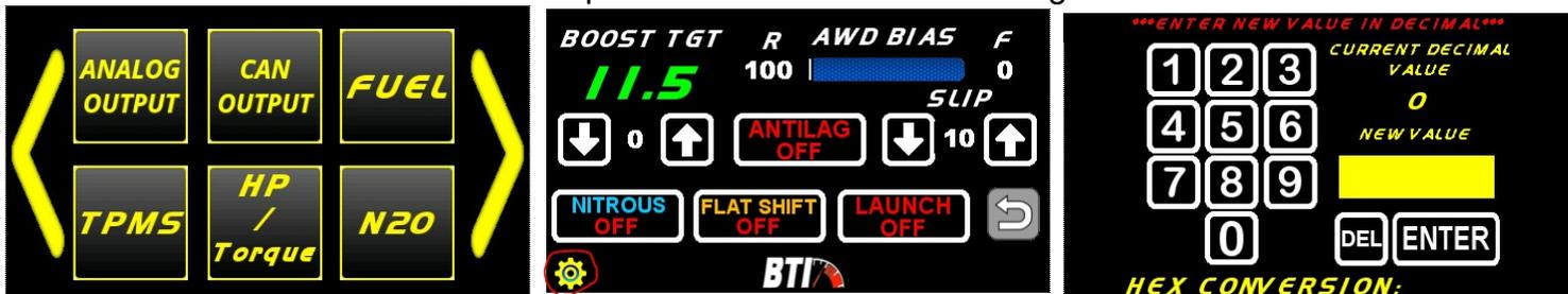
**Pro Tip:** Note that the CAN Message ID is entered into the gauge as a DECIMAL value with a HEX conversion shown at the bottom. The Address listed in the MaxxECU software is shown in HEX.
